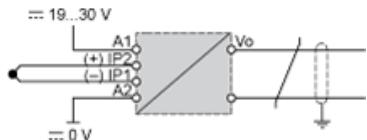
The input, output and power supply lines must be kept away from the power cables to avoid effects due to induced interference.
